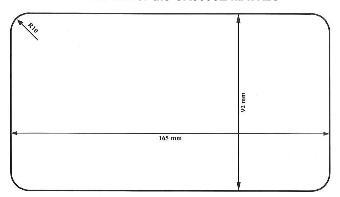
Use this template to mark the location where the rectangular hole for the flush mount is to be cut.
